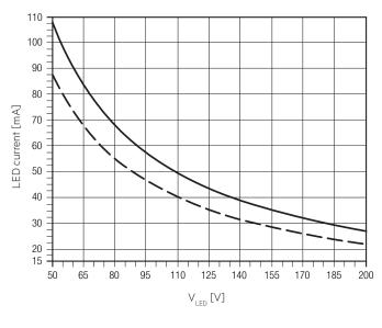
LED current at nominal battery voltage and min. battery discharge current
