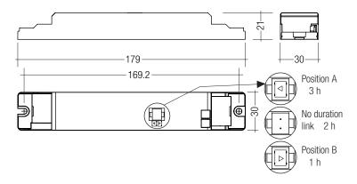
Note: LED Driver supplied with duration link in 3 hours position. Duration link must be set before battery and mains connection. The EM converterLED PRO 135 NiCd is supplied without a duration link. The duration is set to 3 hours and cannot be changed.
