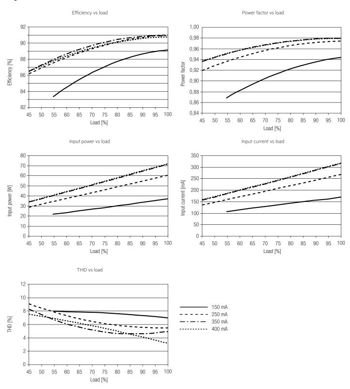
100 % load correspond to the max. output power (full load) according to the table on page 2.
